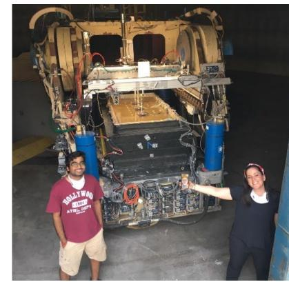
Above: The stress beneath a 50m-tall embankment at 1g is the same as the stress beneath a 0.5m-tall embankment at 100g, increasing similarity in behavior.
