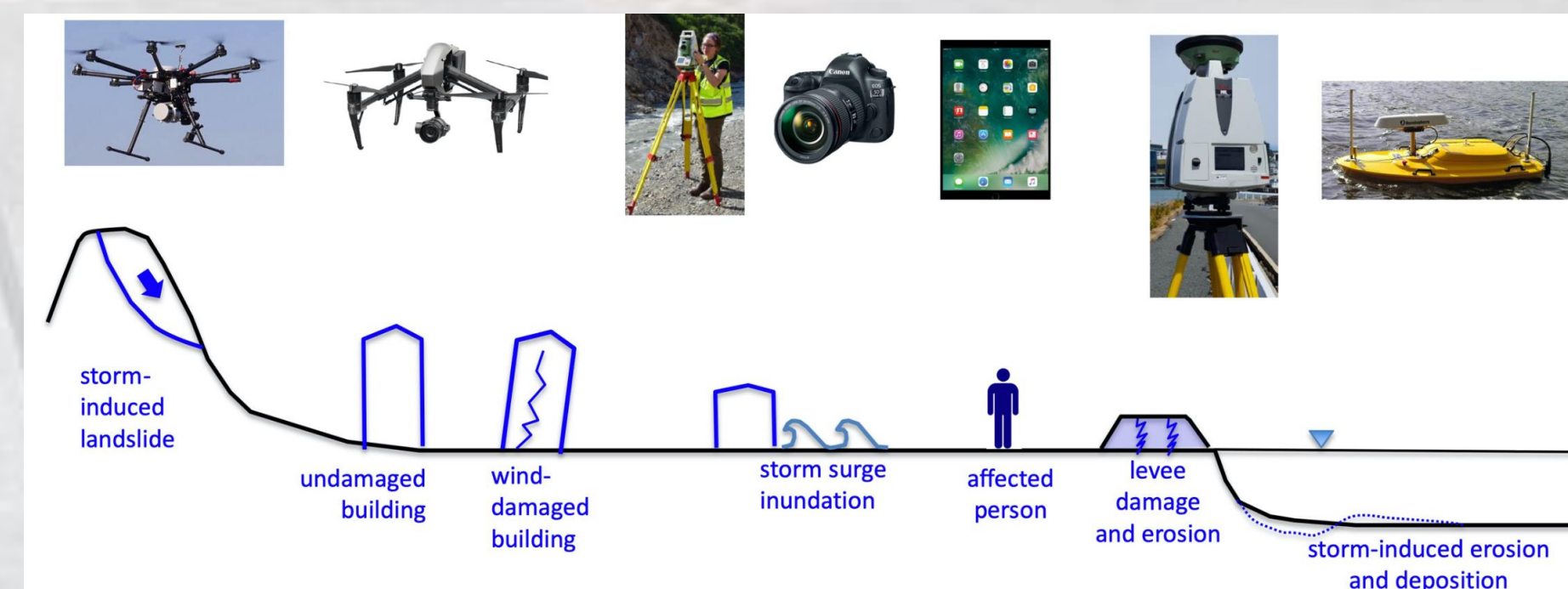
Fig. 3: RAPID Facility Multidisciplinary and Multi-Scale Data Collection (Berman et al. 2020)
