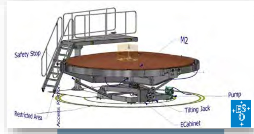
Large Mirror Washing & Stripping
