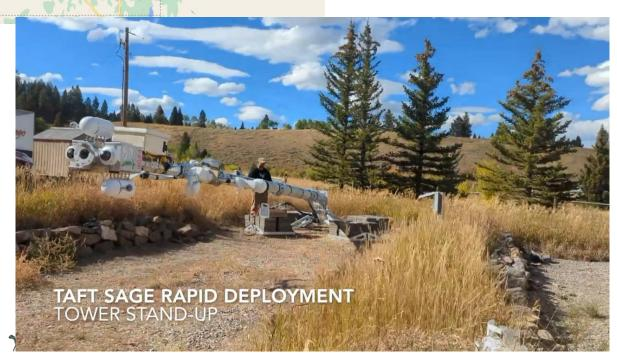
**Sensors:** Sage node with cameras, microphone, TPH, precipitation, dust and thermal camera.
