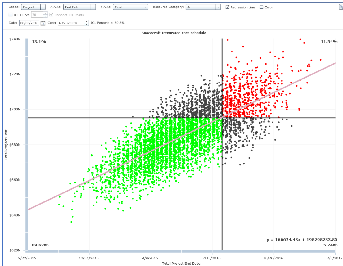
Figure 6.2.8-3 Time-Cost Scatter Diagram: Each data point represents one realization of the simulation
