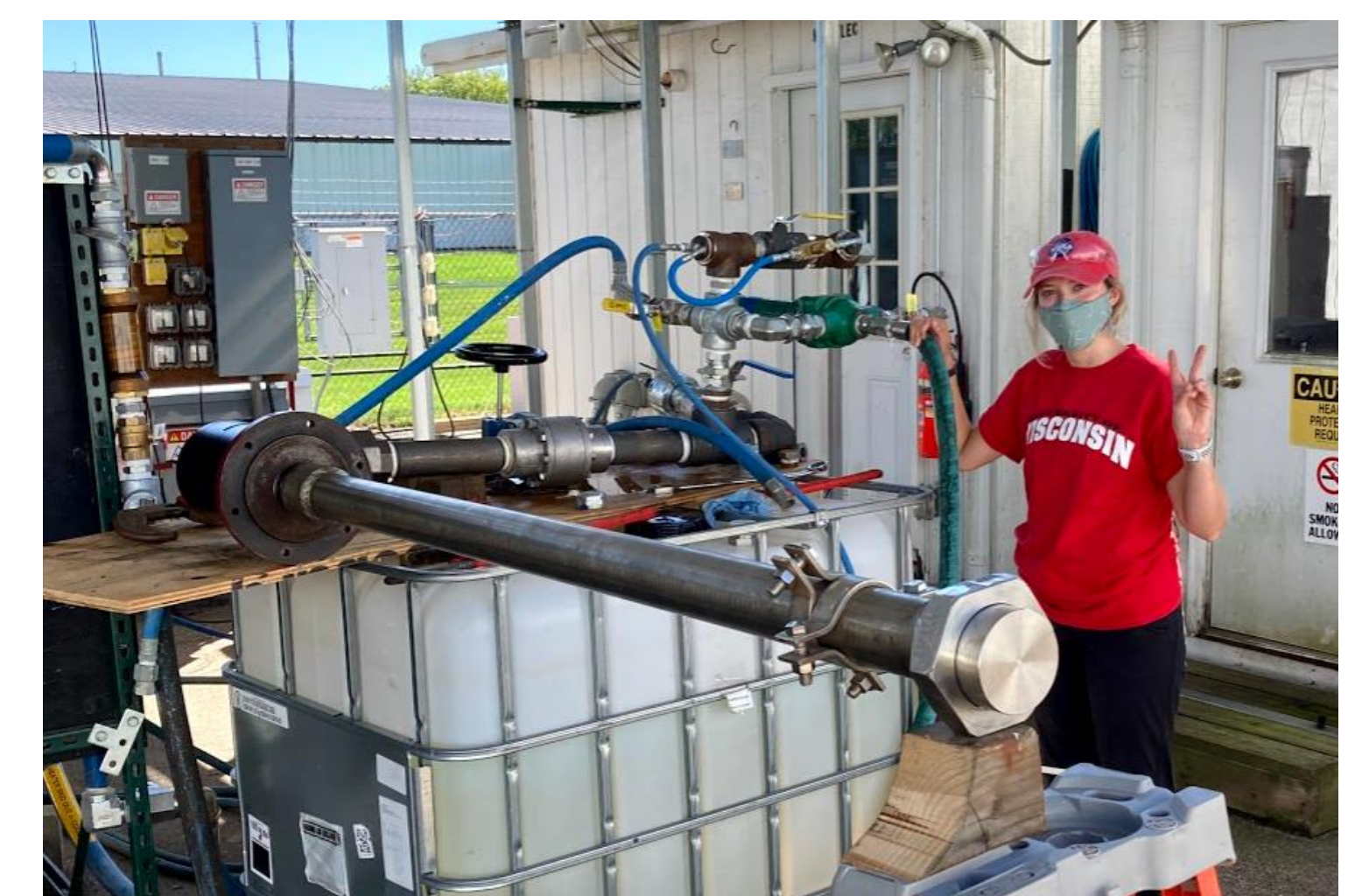
Pressure testing Main Supply Hose Reel plumbing assembly
